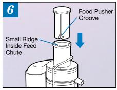
Slide the Food Pusher down the Feed Chute by aligning the groove in the Food Pusher with the small ridge on the inside of the top of the Feed Tube.
